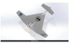
The Indian kamikaze drone will be around 2.8 meters long with a wingspan of 3.5 meters.
